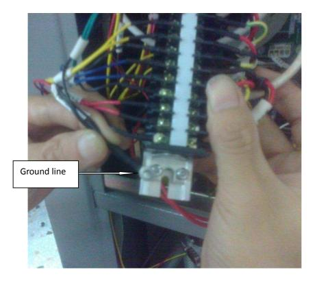
e. Put the terminals on the left of board fixtures (it can not be fixed), then fix the transformer and electron tube socket.
