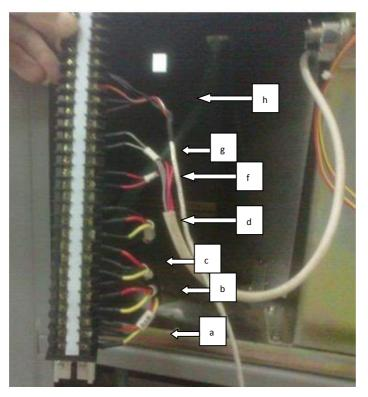
c. The new circuit components which need to put into the upper left corner of instrument as picture. (All connection line include j(1),g(1),f(1),h(1),i(1))
