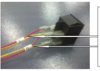
Please note: the bottom is input port"0", and the top is output port"1". The same color line is on the same side.
