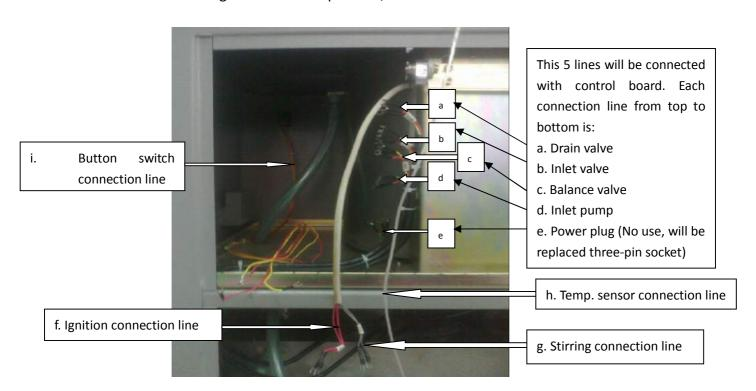
c. Up out of the terminals from the fixed plate after taking out the connection line. (The terminals will be retained to update equipment, The other part will be
